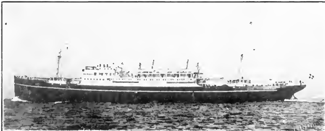
Ms. Amerika, first vessel fitted with Burmeister and Wain double-acting, 2-cycle engines, set an overall fuel consumption of 0.365 pound per brake horsepower.
